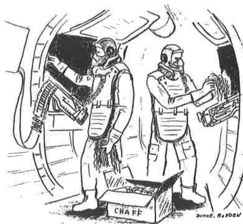
NEAR START OF BOMB RUN THE WAIST GUNNERS WOULD THROW OUT THE "CHAFF". IT LOOKED AND FELT LIKE CHRISTMAS TREE TINSEL, IT FLOATED DOWN AND FOULED UP THE GERMAN GROUND RADAR USED WITH ANTI-AIRCRAFT GUNS. (FLAK GUNS)
