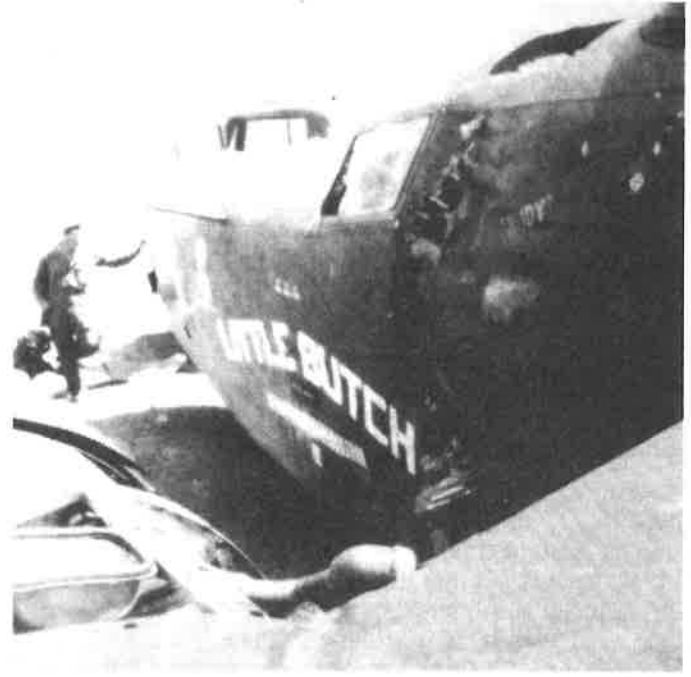
"Little Butch" - Note Gash Where Prop Blade Entered Flight Deck
